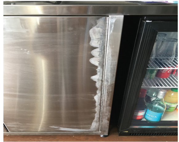
Extreme example of staining due to the weld cleaning solution residue not being completely removed/neutralised
