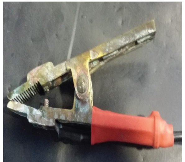
Copper phosphate (a blue coloured di-electric) produced from the clamp not being washed down. This will corrode the clamp teeth and cable lug which can lead to intermittent connection (no power output).
