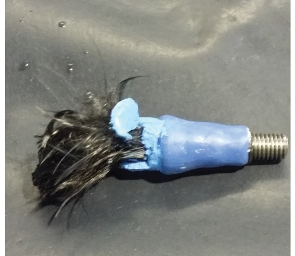
Copper phosphate (a blue coloured di-electric) produced from the brush not being washed down. This will corrode the brush lug and also the thread which can lead to intermittent connection (no power output).
